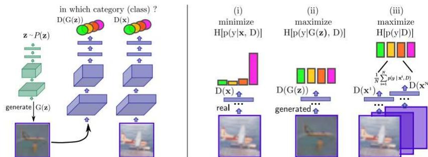
Figure 3. CatGAN image processing and optimization principle
